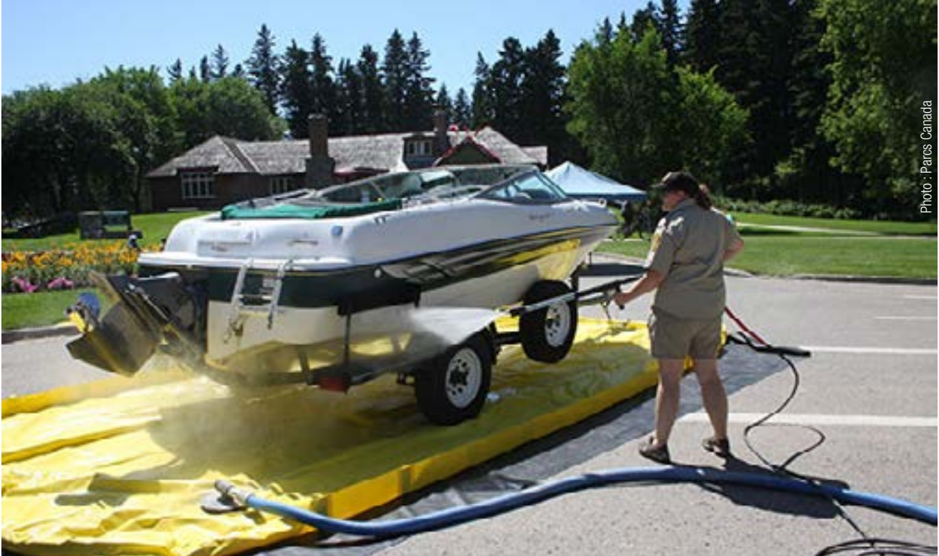
Use of a membrane to recover waste water from a watercraft decontamination station © Parcs Canada
